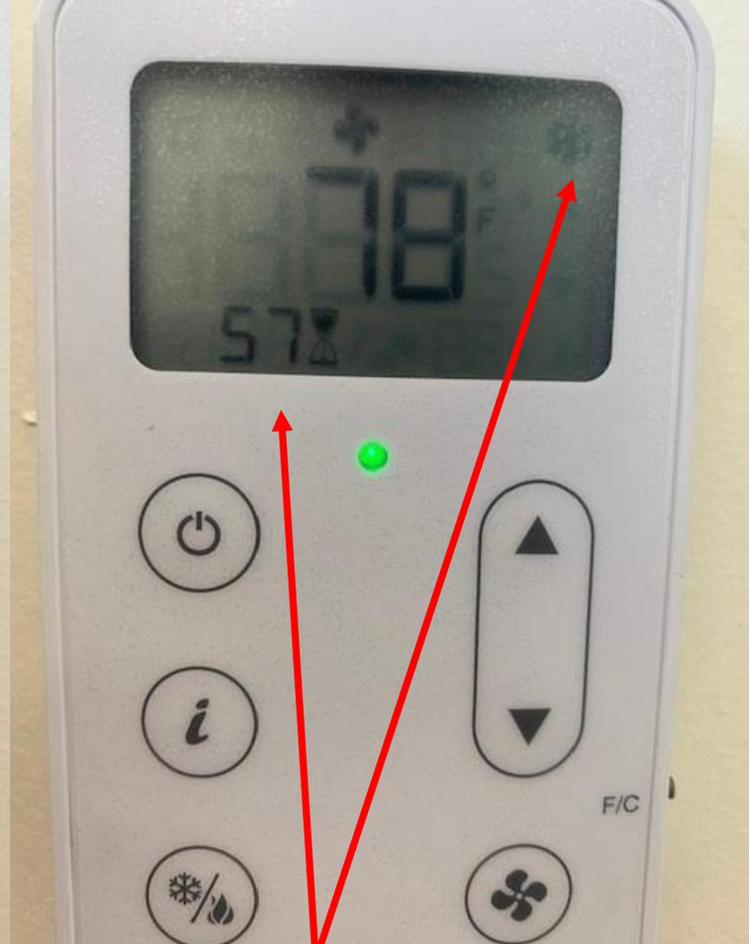
After several seconds, the screen will revert back to the room temperature and the amount of time the unit will be in occupied mode. After several more seconds, the snowflake icon will appear. The unit is now in cooling mode.
